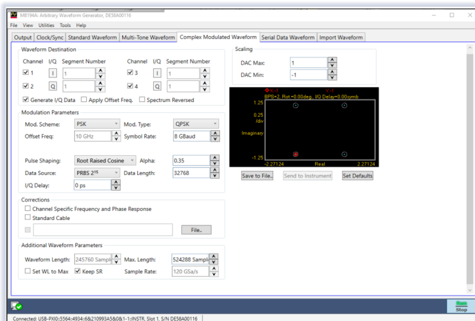
Reference Settings for the free Keysight “IQ Tool” to generate a DP-QPSK Signal
